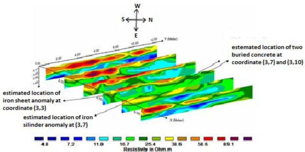
Figure 6. Vertical cross section (y-z) arranged horizontally
