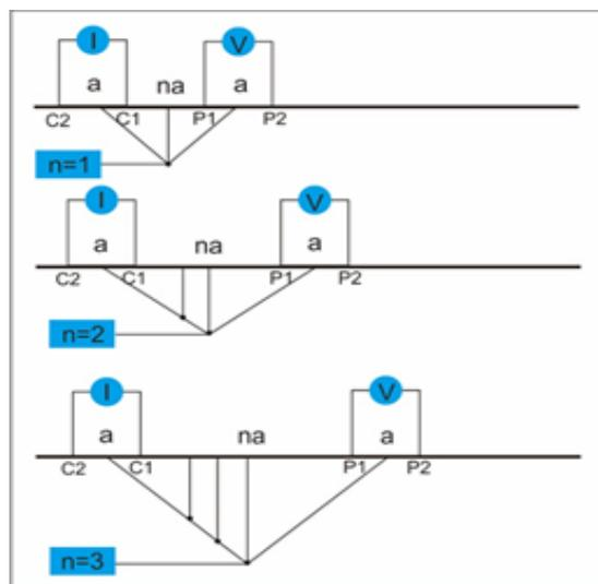
Figure 2 Dipole-Dipole Configuration[12]
